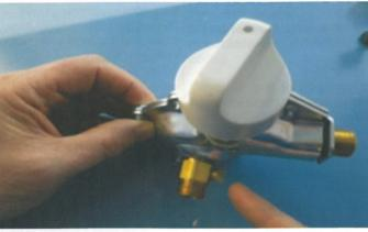
The finger is pointing at the drain plug in the brass body of the cold water inlet at the bottom of the boiler. This drain plug should be removed, taking care to retrieve the plastic washer.
