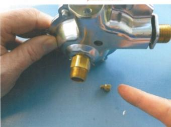
The drain plug has been removed but the washer is still adhered to the brass body.
